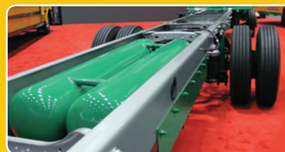
2-tank LPG system offers an estimated 300-mile range with a 70-gallon capacity.
